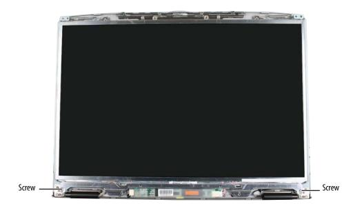
**10** Remove the six screws connecting the LCD panel to the LCD panel assembly.
