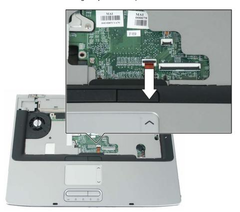
**9** Remove the four screws from the top of the palm rest.
