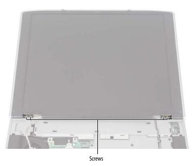
**9** Lift the LCD panel assembly away from the notebook. The LCD panel assembly is now completely detached from the notebook.
