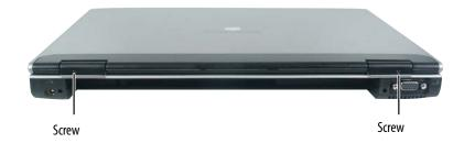
4 Insert the small flat-blade screwdriver or non-marring tool under the bottom each LCD panel hinge and gently pry it up.
