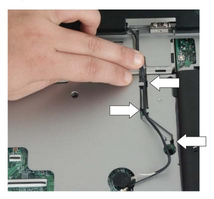
12 Slide the LCD video cable under the retaining clips, then plug the LCD video connector into the notebook.
