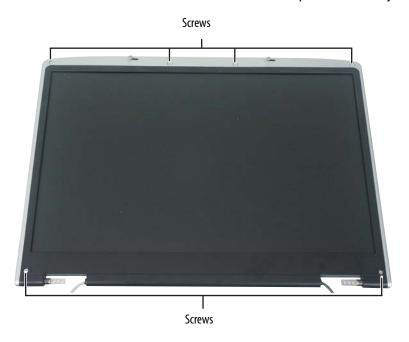
8 Carefully separate the front and back of the LCD panel assembly.
