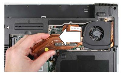
7 Unplug the old cooling fan, then remove the cooling assembly.
