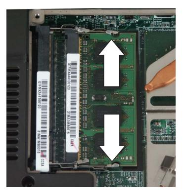
6 Pull the memory module out of the slot.
