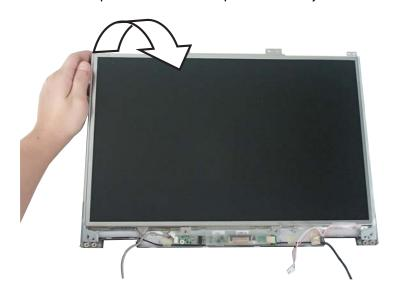
12 If you are replacing the LCD panel into an existing lid and you need to transfer the existing LCD panel inverter to the new panel, unplug both cables from the inverter, then plug them into the new LCD panel.
