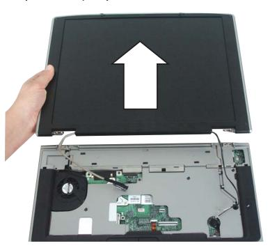
**10** Place the new LCD panel assembly onto the notebook, then replace the four hinge screws.
