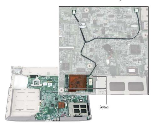
**10** Lift the modem from the system board.
