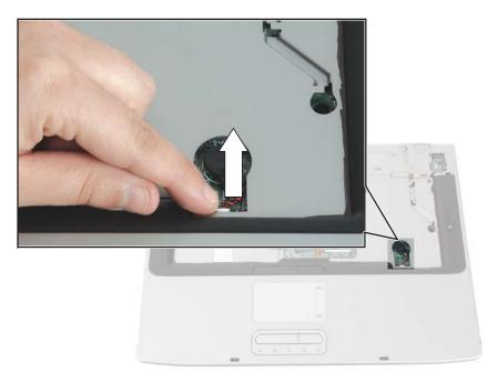
Use only CMOS batteries designed for your Gateway notebook. The non-conductive sleeve and wires are not reusable.
