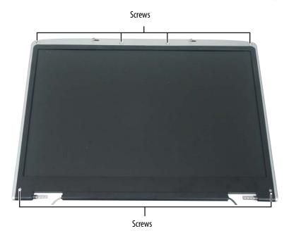
**5** Carefully separate the front and back of the LCD panel assembly.
