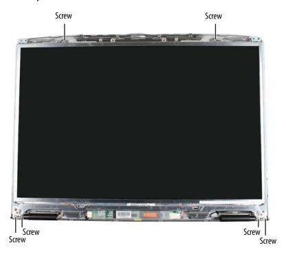
11 Remove the LCD panel from the LCD panel assembly lid.
