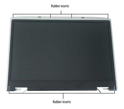
4 Remove the six screws from the front of the LCD panel assembly.
