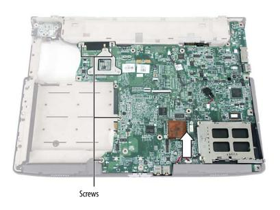
17 Turn the system board over and disconnect the external video board from the old system board and connect it to the new system board.
