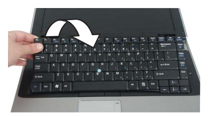
11 Carefully rotate the keyboard toward you so it lies **keys-down** on top of your notebook. Be careful not to damage the LCD panel.
