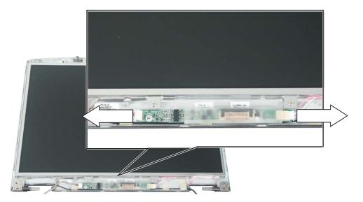
13 Place the new LCD panel into the existing LCD panel assembly lid. -OR-
