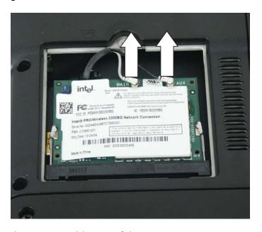
4 Move the antenna cables out of the way.
