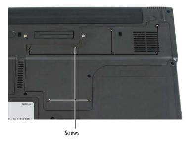
**4** Use the thumb notch to lift the memory bay cover, then remove it. Be careful not to break off the tabs located on the end of the cover opposite of the thumb notch.
